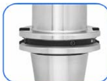
- True Dynamic Balance HPI ER collet chucks are dynamically balanced not production balanced. Standard = G6.3 @ 10,000-12,000 rpm SG Series = G2.5 @ 20,000 rpm
